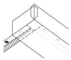
4. Adhere membrane to Stripbond Tape and apply up wall to approved termination. Cut and install membrane at corner as shown. Roll top surface of membrane with a 5 cm silicone roller over tape. Heat weld the membrane overlap.
