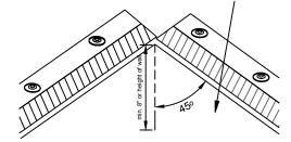
Position membrane at corner and cut 45 degree angle along dashed line as indicated.
