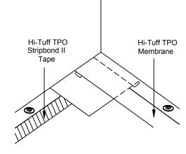
3. Fold membrane back onto itself and apply Primer/Adhesive to back surface of Hi-Tuff TPO membrane where it will contact the Stripbond II Tape. Apply adhesive to wall substrate.
